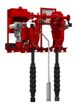
The new 1KVT fire-fighting pump sets with diesel engine or electric motor assembly, ideal for automatic sprinkler systems and/or hydrants of commercial buildings, are manufactured using vertical turbine pumps, in accordance with article 10.6.1 of UNI EN 12845 standards.
