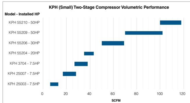
\* HP shown is the maximum installed motor HP based on standard running operating conditions at maximum speed. Performance based on 15°C (60°F) water as the service liquid.
