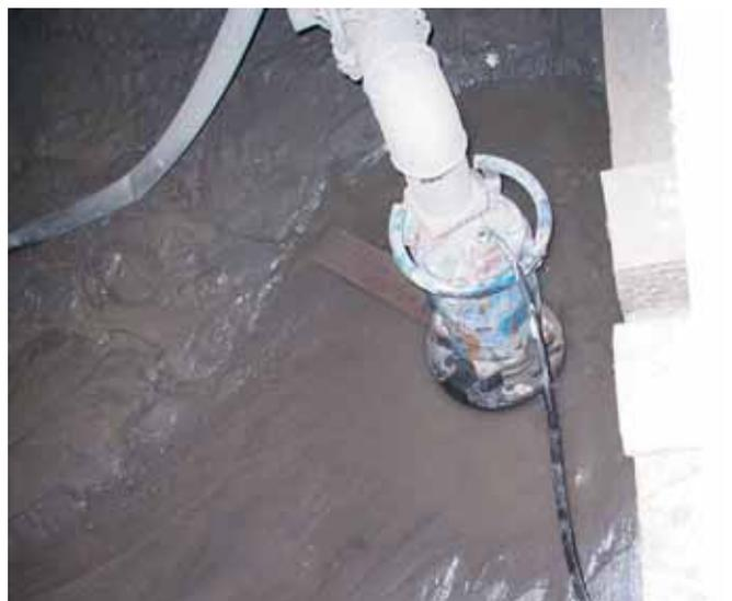
In the event of abrasive and corrosive utilization, stronger wear and tear will take place naturally in certain components. With regards to the above application wear and tear can take place mainly in impeller, agitator, suction plate, shaft sleeve, oil ring, mechanical seal, pump casing, strainer, motor casing and discharge coupling. Depending on the working conditions the lifetime of those parts might vary significantly and can be shorter than the legal warranty period.
