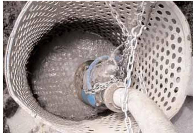
In the event of abrasive and corrosive utilization, stronger wear and tear will take place naturally in certain components. With regards to the above application wear and tear can take place mainly in impeller, agitator, suction plate, shaft sleeve, oil ring, mechanical seal, pump casing, strainer, motor casing and discharge coupling. Depending on the working conditions the lifetime of those parts might vary significantly and can be shorter than the legal warranty period.
