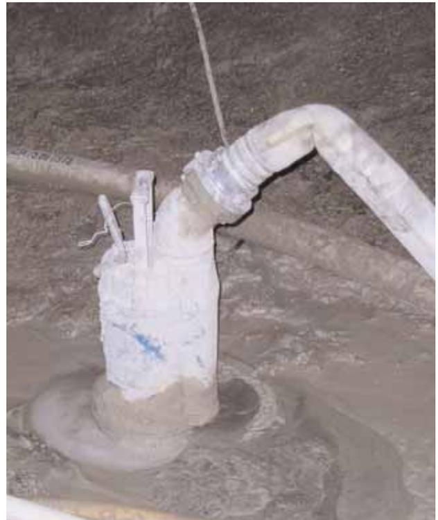
KTZ32.2 in use for drainage at the working face
