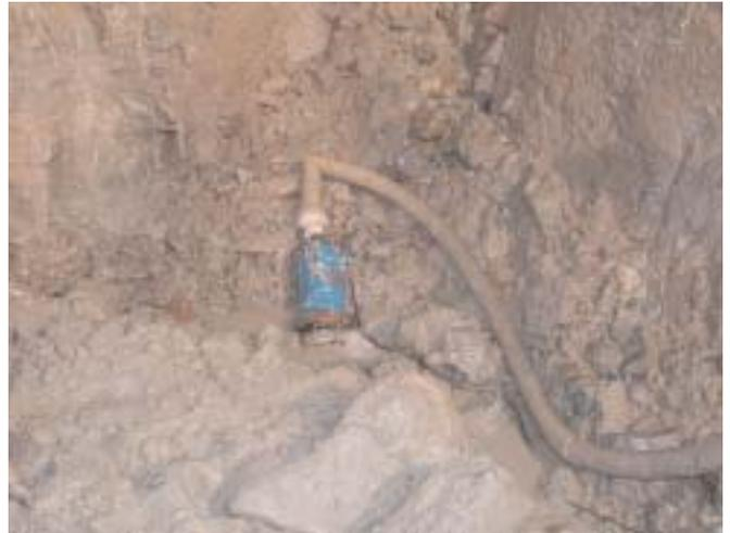
In the event of abrasive and corrosive utilization, stronger wear and tear will take place naturally in certain components. With regards to the above application wear and tear can take place mainly in impeller, suction plate, shaft sleeve, oil ring, mechanical seal, pump casing, strainer, motor casing and discharge coupling. Depending on the working conditions the lifetime of those parts might vary significantly and can be shorter than the legal warranty period.
