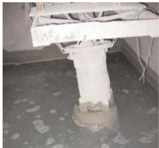
In the event of abrasive and corrosive utilization, stronger wear and tear will take place naturally in certain components. With regards to the above application wear and tear can take place mainly in impeller, agitator, suction plate, shaft sleeve, oil ring, mechanical seal, pump casing, strainer, motor casing and discharge coupling. Depending on the working conditions the lifetime of those parts might vary significantly and can be shorter than the legal warranty period.
