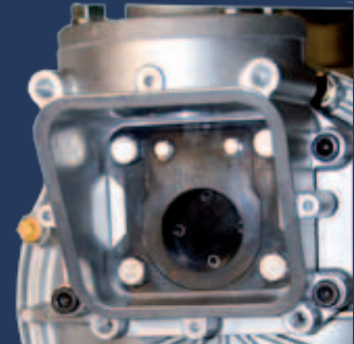
Only 4 bolts to access flap valves
