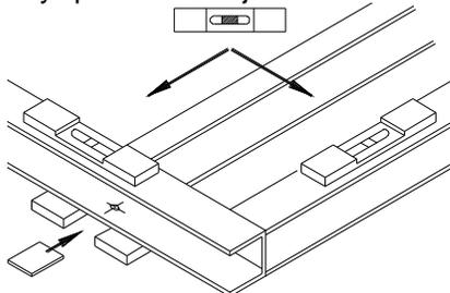
Level with shims between baseplate and packing pieces.
