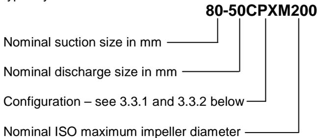
The typical nomenclature above is the general guide to the CPXM configuration description. Identify the actual pump size and serial number from the pump nameplate. Check that this agrees with the applicable certification provided.
