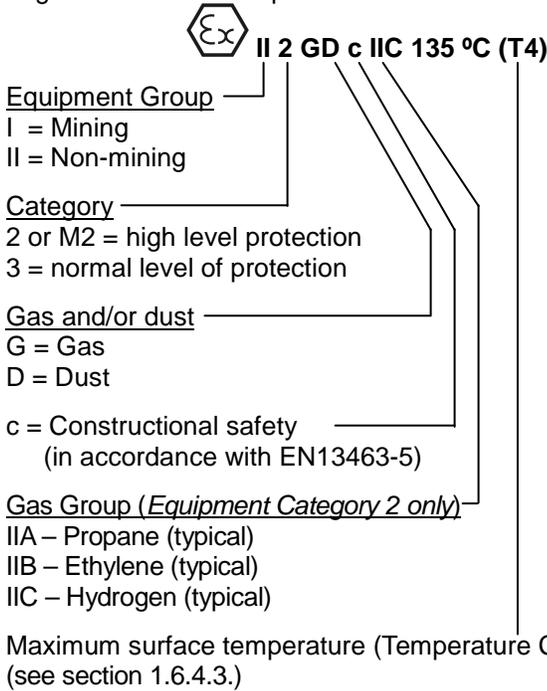
**1.6.4.3 Avoiding excessive surface temperatures**
