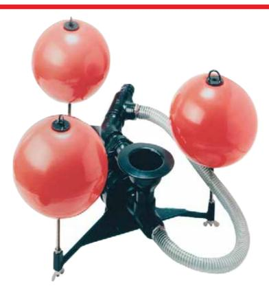
A bypass attached to the discharge opening recycles part of pumped water to the intake to generate a jet flow. An ejector effect produced by the jet flow, generates suction power in the collection cup (Intake).
